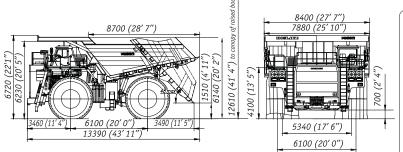
\*Overall dimensions are specified for basic kitting-up of the dump truck
